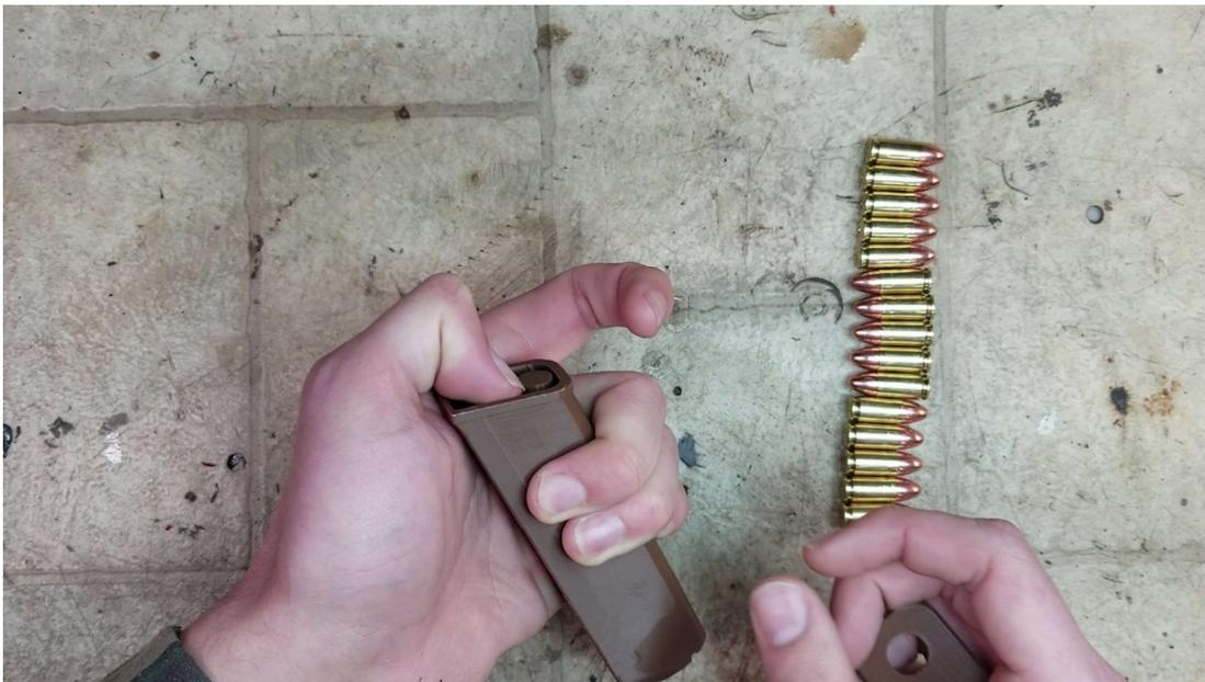
Slide the baseplate onto the lip edge at the bottom of the magazine. The REAR of the baseplate (the side with the open end) will slide onto the FRONT of the magazine (where the magazine is curved).
