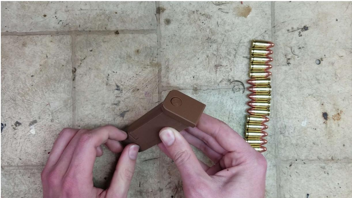
In order to disassemble your magazine, you need only take a cartridge, punch, or other sort of tool (even your pinky finger) and push the locking tab inwards (compress the spring) while pushing the baseplate forwards. After removing the baseplate, you can disassemble in the reverse order that you assembled.
