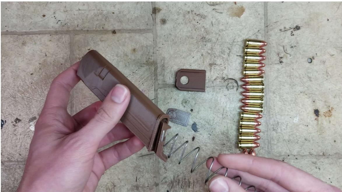
After inserting the spring and follower, take your locking tab. You will be using the locking tab to depress the spring into the magazine. Make sure the front of the locking tab (the angled side) is towards the front of the magazine. Make sure that the round peg on the locking tab is facing AWAY from the magazine spring.
