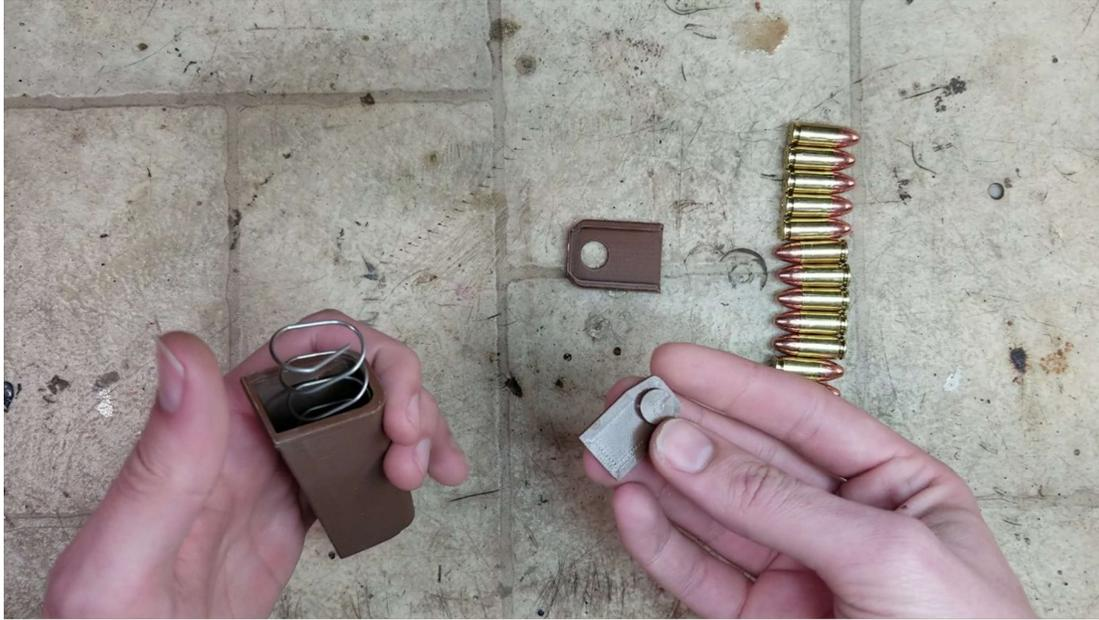
While holding down the magazine spring using the locking tab (again, make sure that the round peg is facing AWAY from the magazine spring), grab your baseplate. This is what things should look like before your baseplate is installed, while you are compressing the magazine spring with the locking tab.
